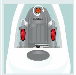
During normal circulation of solution during descaling or chemical cleaning, both ISOLATING VALVES 1 & 2 should be pointing downward.
