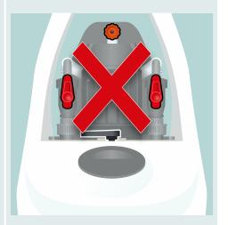
During discharging only one ISOLATING VALVE should be rotated into the discharge setting.
