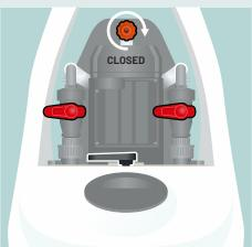
The closed isolating valves position is used when initially setting up the pump, after finishing the flush or if the pump is turned off for any reason.
