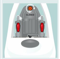
During normal circulation of water through the system during a power flush, both ISOLATING VALVES 1 & 2 should be pointing downward.
