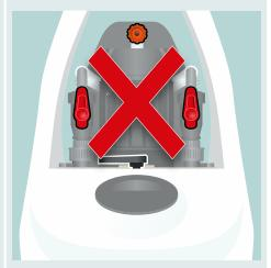
During discharging/dumping, only one ISOLATING VALVE should be rotated into dumping position.
