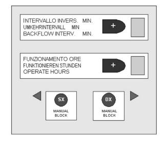
alternately will reverse the flow direction of the pump.
