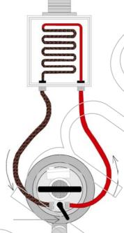
This reduces the descaling time considerably, and is more effective in flushing out any solid matter, which will accumulate on the circumference of the base of the tank. By attacking scale from both sides it is also possible to clean piping which is almost totally obstructed.
