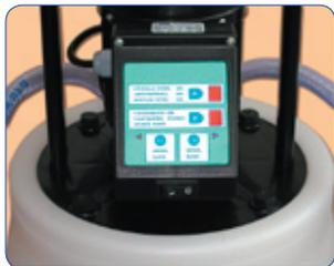
The Scalebreaker C15 AFR pump has an electronically controlled flow reversing device, which enables the pump to be left unattended during the descaling process. The automatic valve may be set to control overall running time, and the frequency of flow reversal.
