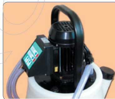
In use, the tank is filled with descaling chemical, connections are made to the water inlet and outlet of the equipment to be descaled or flushed, and the pump switched on until cleaning is complete.
