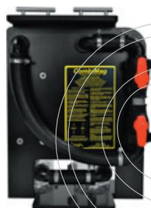
The CombiMag Twin filter is installed in line with the power flushing pump. The cyclone construction directs contaminated water through a powerful magnetic field, such that even the smallest of particles are retained on the central magnets, from which they may be easily cleaned during and after power flushing.
