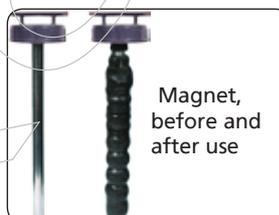
The debris retained on the magnet is an impressive visual aid. It demonstrates to property owners what has been removed from the system, confirms the need for the power flush, and demonstrates
