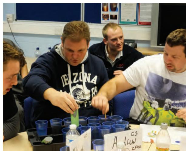
Testing the waters: Using a turbidity tube (left), a TDS meter (centre) and a pH meter and paper (right) to ensure the system has been properly cleaned
