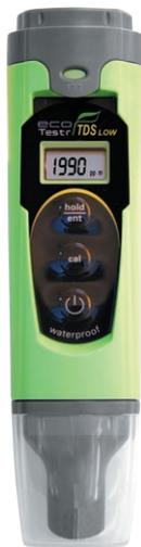
Before first use of the Eco Testr, soak sensor for 2 minutes in alcohol to remove oils. Rinse in clean water.
