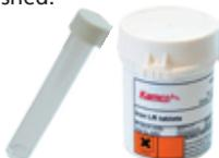
Mains water often contains iron, although at levels of less than 1 mg/l. A test reading of more than 1 mg/l above the mains water indicates that corrosion is taking place (even though water drawn from the top of a radiator may be clear), and the system should be power flushed.
