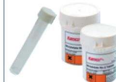
The test measures the molybdate content within a heating system. 330 mg/l (ppm) molybdate is the optimum treatment level of 1% Systemsafe-DM by volume, and 100 ppm for 0.5% Systemsafe DM Concentrate.
