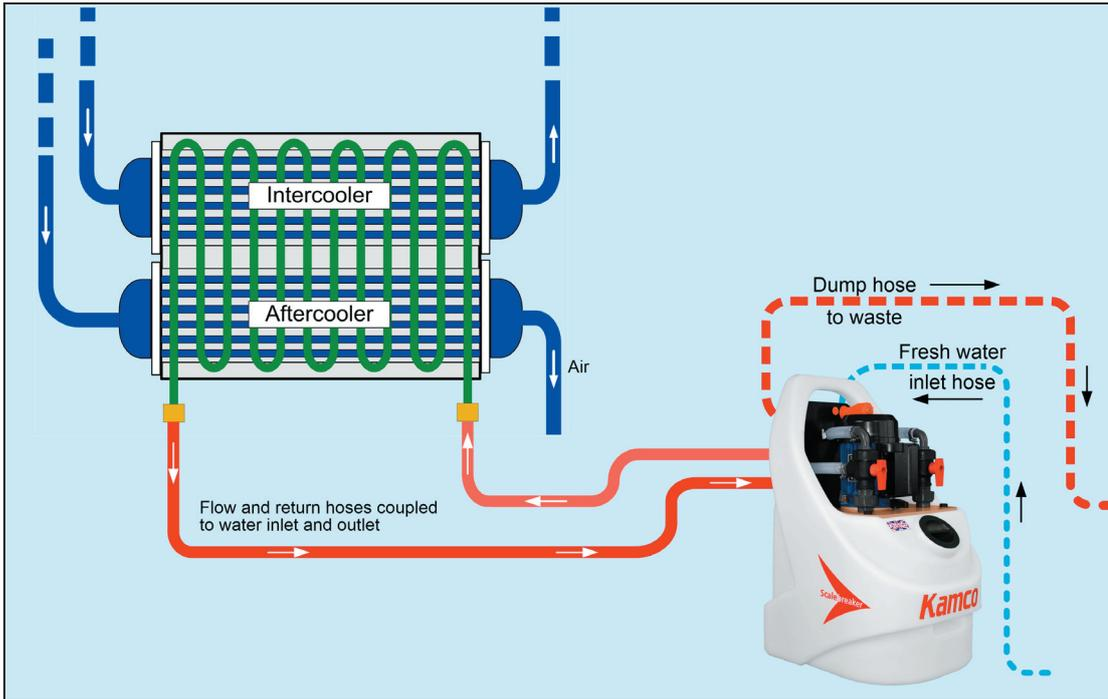
Scalebreaker C40 FWF with fresh water flushing facility
