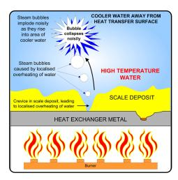
high temperature zone to cooler areas, the temperature falls back below the boiling point of water, and the bubbles collapse and implode to give unpleasant and irritating noises.
