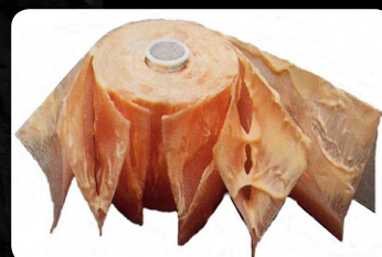
Fuel filter blocked with precipitated wax
